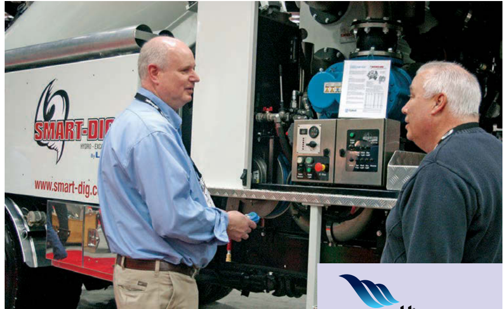
Mike Fenneman, left, owner of LMT Inc., discusses the features of the HX-4000 hydroexcavator with a WWETT Show attendee. The modular unit can be mounted on chassis options from a variety of makers.
