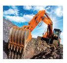
durable hydraulic pumps provide great lift capacity and swing torque to boost productivity. The larger pumps, a heavy operating weight and a redesigned boom and arm allow the operator to maximize efficiency by using a larger bucket.
