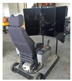
This Great Excavations remote control workstation allows operators to safely run their excavators and other heavy equipment from a remote location.
