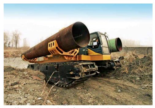
An amphibious pipe carrier removes large pipe from a work site. It can be run remotely from shore, keeping operators out of danger.
