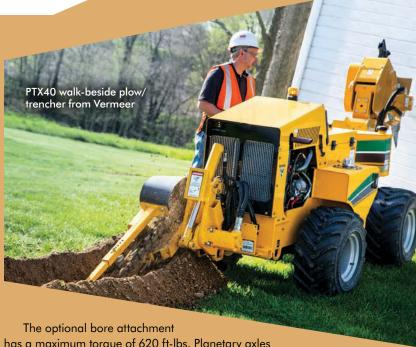
has a maximum torque of 620 ft-lbs. Planetary axles reduce stress and torque on the drivetrain.
