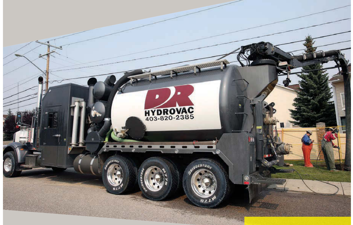
DR Hydrovac owns four Tornado F4 Slope hydroexcavators.
