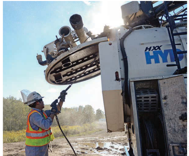
Canyon Environmental operator Jordan Glimm cleans a Vactor HXX hydroexcavator after dumping its used content at the company's debris yard in Mansfield, Pennsylvania.
