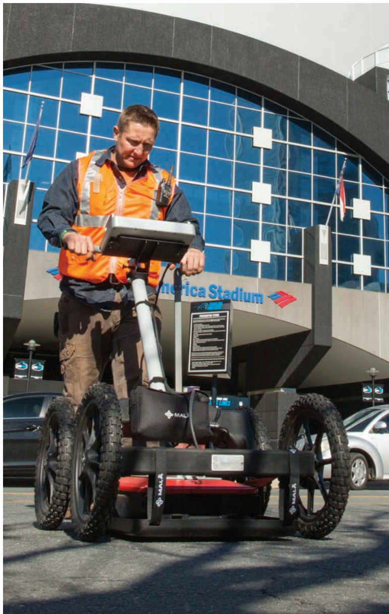
Matt Bellmann made his dream of owning a business a reality. Here he uses a ground-penetrating radar unit (MALA) to locate utilities.
