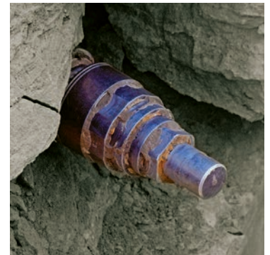
Stationary heads are used for soft soils and reciprocating heads for harder soils.
