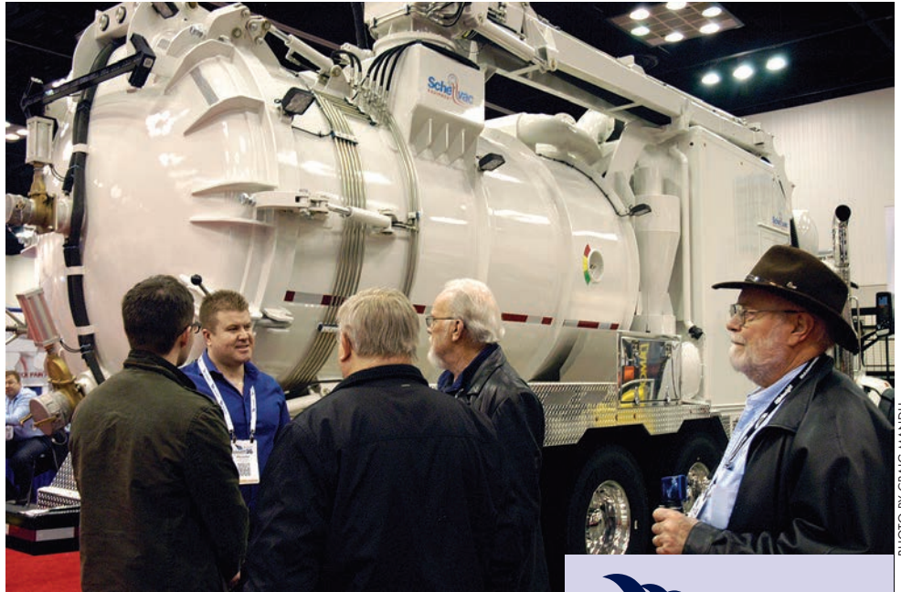
Alexander Scheller, president of SchellVac Equipment, discusses his SCH VT 2600 tri-drive hydroexcavator with a group of 2016 WWETT Show attendees. The unit has a large, hoisted 15.5-cubic-yard debris body with full-opening rear doors with hydraulic locks, and is built on a heavy-duty tri-drive, triple-axle system.
