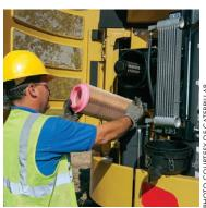
Hydraulic maintenance, engine maintenance, and filter checks are critical to proper care of excavators. Oil and grease checks should be completed on a regular routine.
