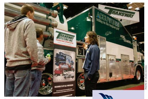
Travis Ouimet, right, parts manager with Transway, discusses the Terra-Vex hydroexcavator with 2016 WWETT Show attendees. The unit's direct-drive blower with transfer case, silencers and water system are contained within an insulated, heated acoustical walk-in enclosure, enabling the unit to be used in subzero temperatures.
