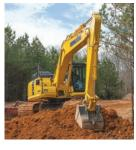
It comes with a viscous fan clutch for improved cooling, three travel speeds, and heavy standard counterweight (9,634 pounds) for improved overthe-front and over-the-side lift capacity.
