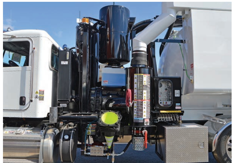
Operators should keep an eye on the hydroexcavation unit's blower sight glass and oil level on every job as part of daily maintenance work.
