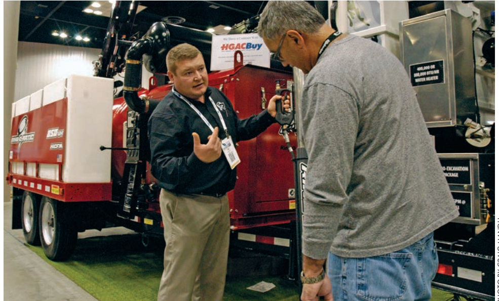
Jim Zylstra, left, Ring-O-Matic’s sales and marketing manager, discusses the HiCFM 850VX trailer-mounted vacuum excavator with a 2016 WWETT Show attendee. Applications include keyholing or potholing buried utilities, cleaning out storm drains and catch basins, drilling fluids, valve boxes, slot trenching, or assisting in environmental cleanup, making it a versatile option for customers looking to complete a wide variety of projects.
