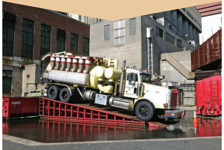
An APC Corporation truck is backed up a ramp to off-load into one of the company's specialized dewatering dump containers.
