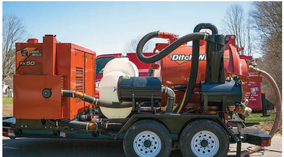
A Ditch Witch vacuum excavator sits on a job site in New Hampshire where a crew is using it with a directional drill.
