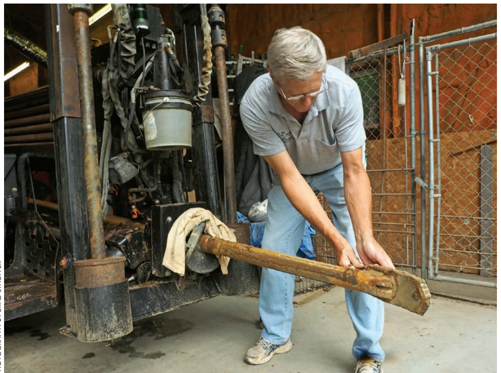
Mid MN Septic Services owner Bob Billiet maintains the beacon assembly on his Ditch Witch JT2020 Mach 1 horizontal directional drill.
