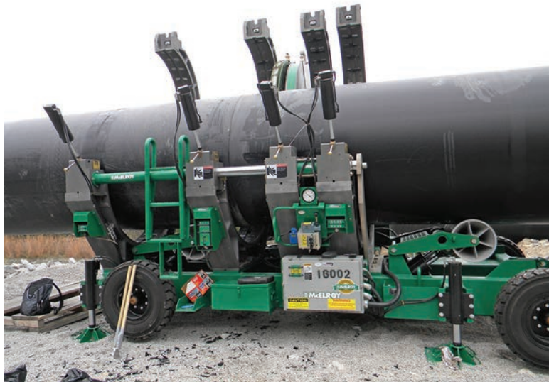
The 1600 fusing machine is the largest made by McElroy.
