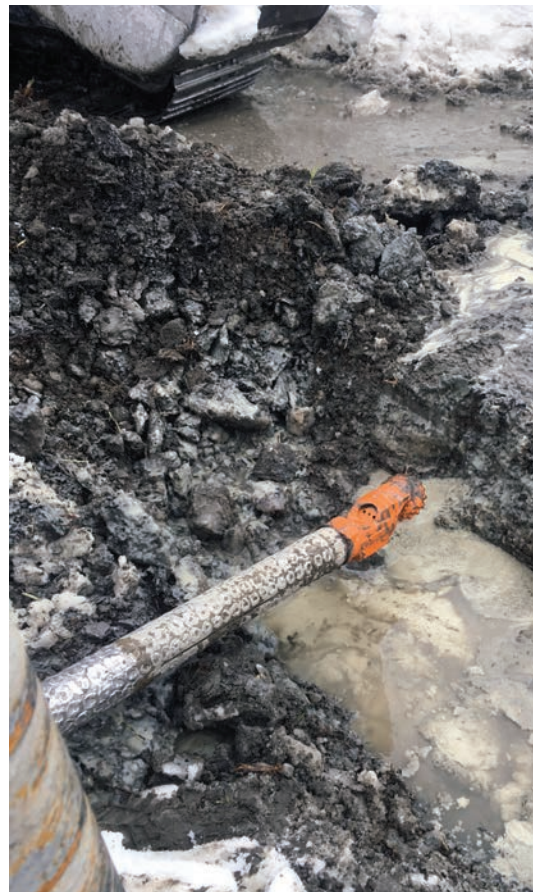
Drillhead's Qui-Kone XL TCI is used in 40,000 psi rock on the north slope of the Brooks Range in Alaska.
