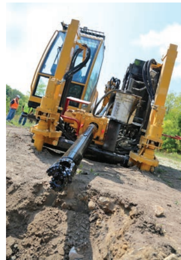
Vermeer introduced the Lance Pro bit at the 2017 CONEXPO-CON/AGG, shown here on the D40x55 directional drill. The bit was first designed for the company's plate family of bits, but it was reinvented as a scoop bit for cobbled rock.
