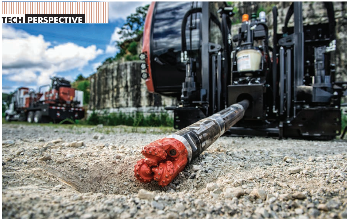
The Ditch Witch RockMaster backreamer with patented edge protection and wear resistance is designed for drilling in rock.
