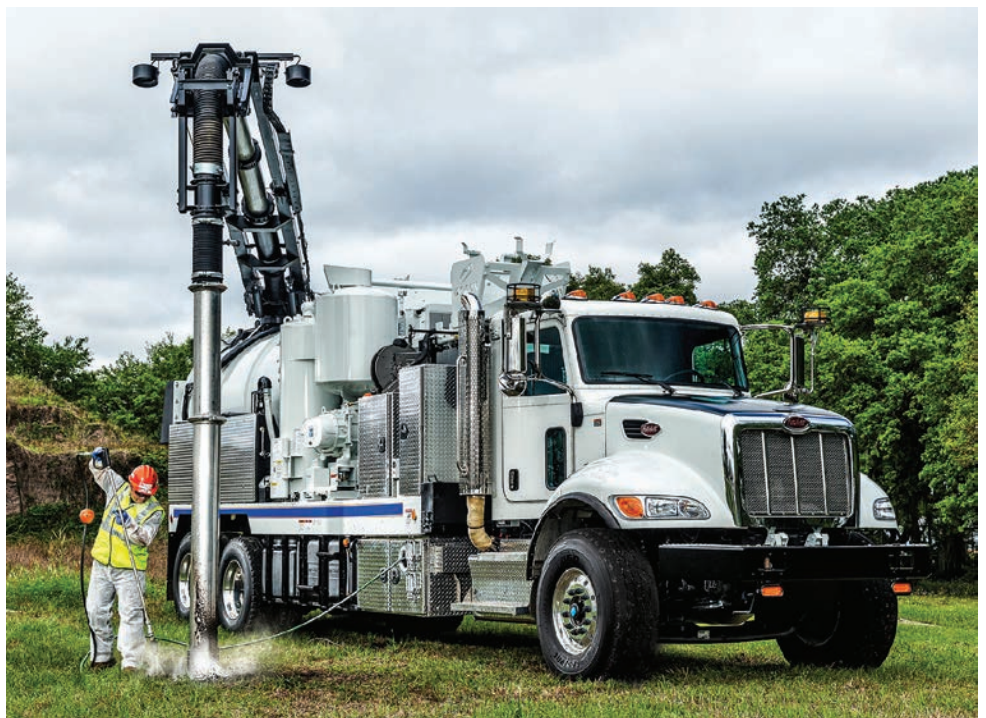
Maintaining hoses, dig tubes and digging wands is essential to keep vacuum excavators working the best they can. Contractors should check over these systems daily to ensure they are in working order.
