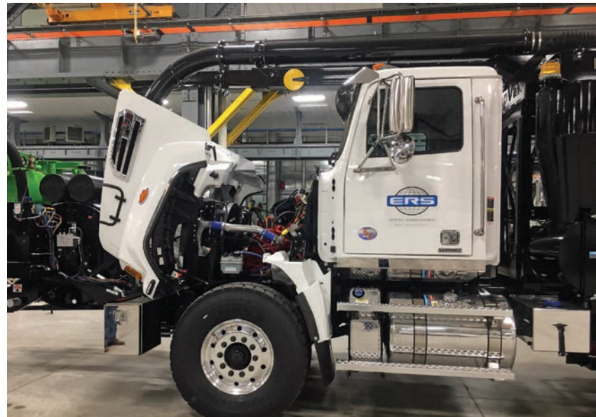
Contractors can maintain the chassis fluids without moving the boom on a GapVax unit.
