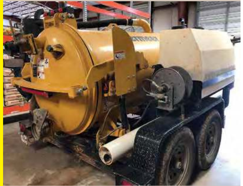
The VX500 vacuum excavator from McLaughlin (owned by Vermeer) is one of Underground Systems' go-to equipment items used on most job sites.
