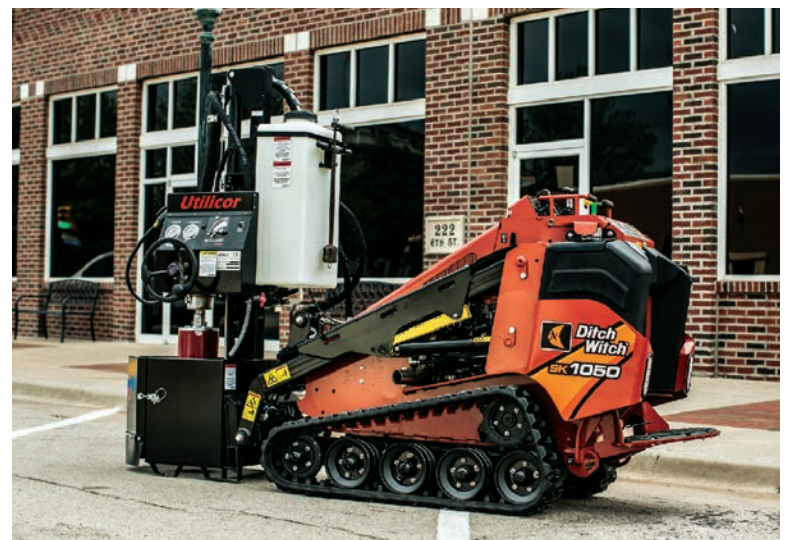
An SK1050 mini skid-steer has a Utilicor Technologies coring attachment installed.
