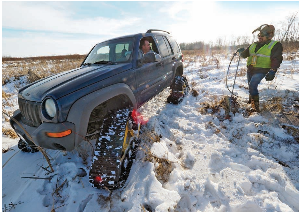
Troy Peterson checks in with Keith Kiehl, who takes a break from potholing a pipeline. Peterson drives a 2002 Jeep Liberty, outfitted with MatTracks EZ HD track conversion system treads.
