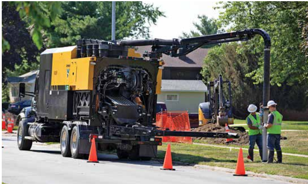
In October, Vermeer unveiled its new Vermeer XR2 vacuum excavator. The unit combines the digging of a vacuum excavator with the ability to separate liquids from solids on the job.
