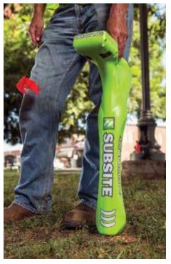
Using a utility locator along with vacuum excavation will help in avoiding damage to buried lines.
