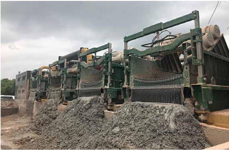
Soil that had just gone through a fluid cleaning system is removed from the system.
