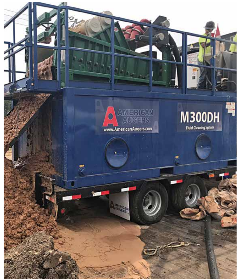
An American Augers M300DH drilling fluid cleaning system sits on a job site. Using a drilling fluid cleaning system allows the crews to reuse the drilling fluid and dry the soil, reducing the need to haul it away.
