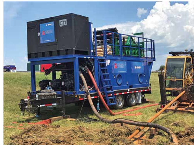
Drilling fluid systems can come in many different size like this smaller M-300D system from American Augers, connected to a directional drill.
