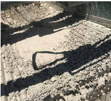
A shaker screen is one of the most important pieces to the drilling fluid cleaning system in HDD operations. They remove solids on the first cut and can dispose of them before going into the fluid cleaning system.
