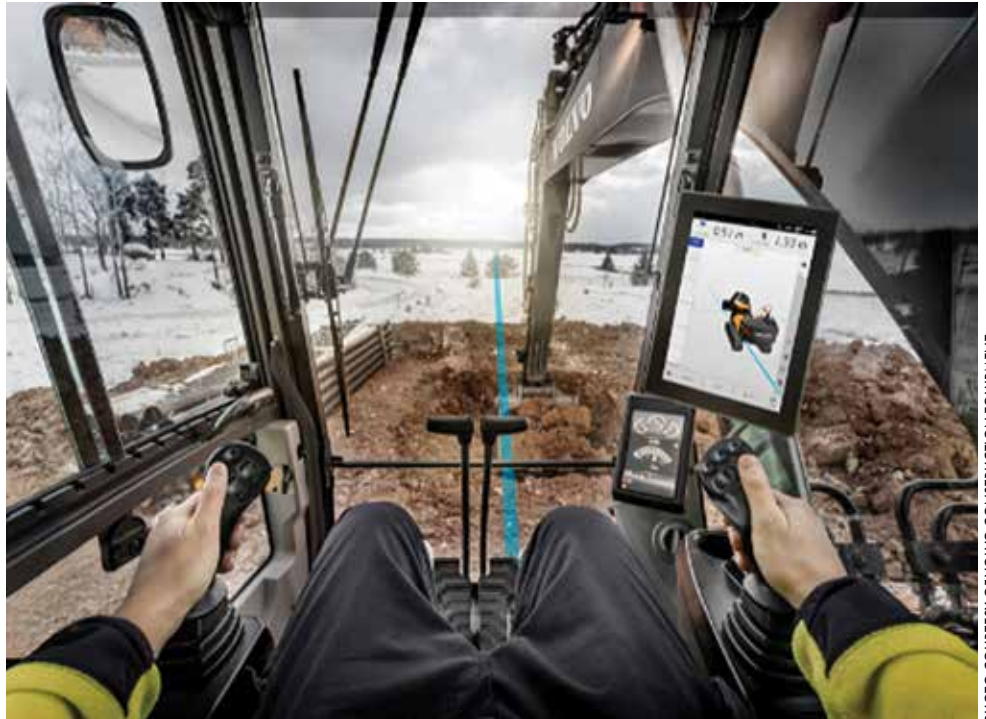
Dig Assist, a system from Volvo Construction Equipment, is standard on the company's 22- to 55-ton excavators. On other models it is an option. The technology lets operators know both visibly and audibly if they are on grade.
