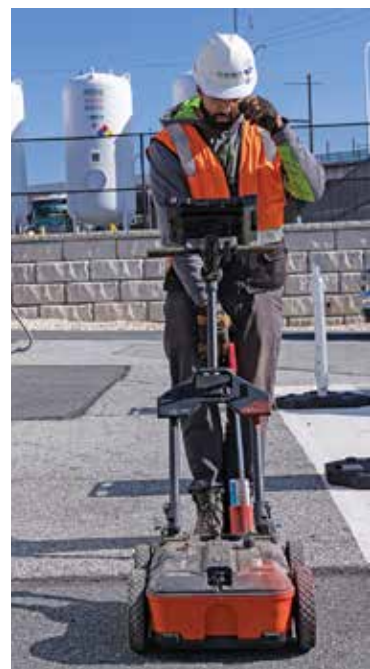
Utility locating specialist Daelvi Garcia uses a UtilityScan (Geophysical Survey Systems) to identify utilities and other objects under concrete and asphalt.
